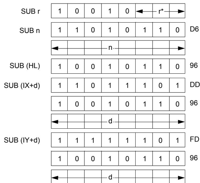
*r* identifies registers B, C, D, E, H, L, or A assembled as follows in the object code field:
