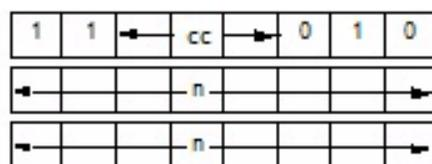
The first *n* operand in this assembled object code is the low-order byte of a 2-byte memory address.
