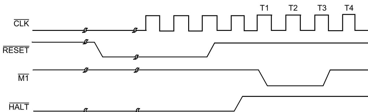
Figure 14. Power-Down Release Cycle, #2 of 3
