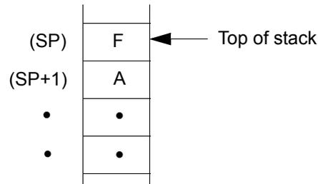
**Figure 36. Example of a 16-Bit Load Operation**
