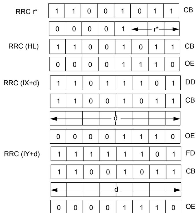
$r$  identifies registers B, C, D, E, H, L, or A assembled as follows in the object code field:
