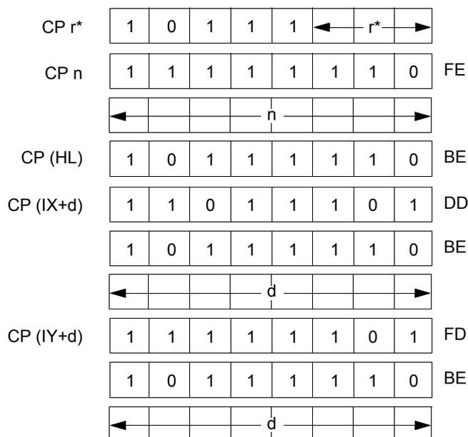
*r* identifies registers B, C, D, E, H, L, or A specified in the assembled object code field, as follows:
