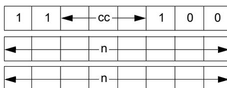
The first of the two *n* operands in the assembled object code above is the least-significant byte of the 2-byte memory address.
