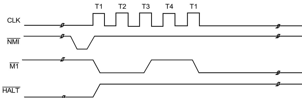
Figure 13. Power-Down Release Cycle, #1 of 3
