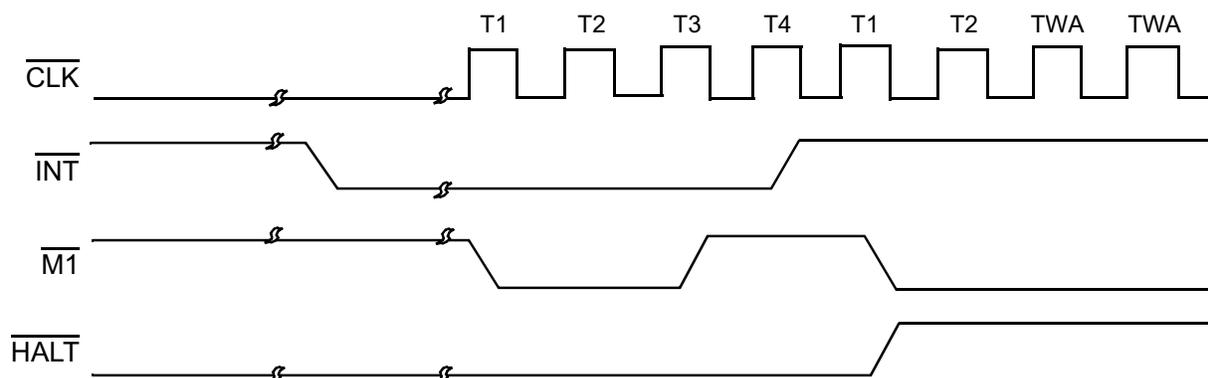
Figure 15. Power-Down Release Cycle, #3 of 3
