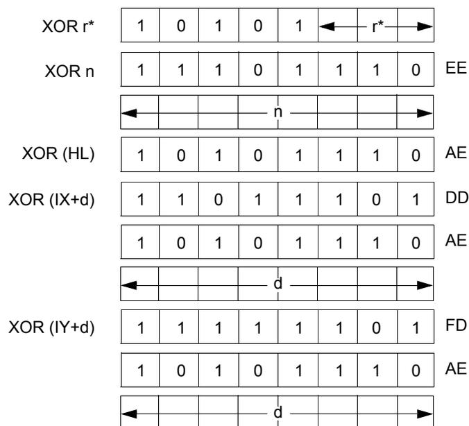
*r* identifies registers B, C, D, E, H, L, or A specified in the assembled object code field, as follows:
